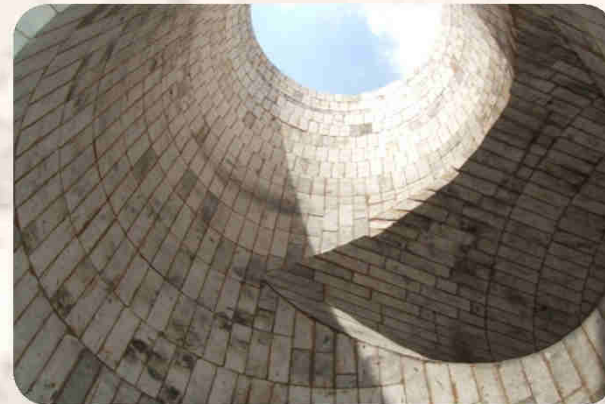
Carbon Black reactor after repair / lined with corundum special bricks LUPUDUR K 99
